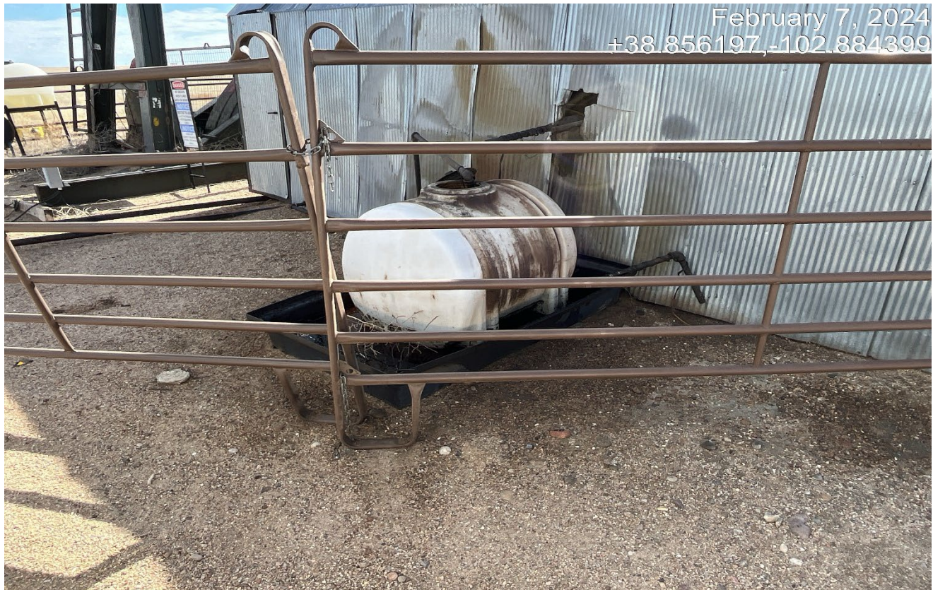
Photo 4. There is oily fluids inside the secondary containment of this white tank. There is oil staining on the ground and the lid is not secured.
