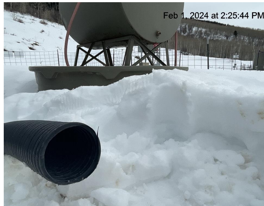
Photo # 5309 Flowline heating insulation open ended/wildlife hazard/available for entry by wildlife
