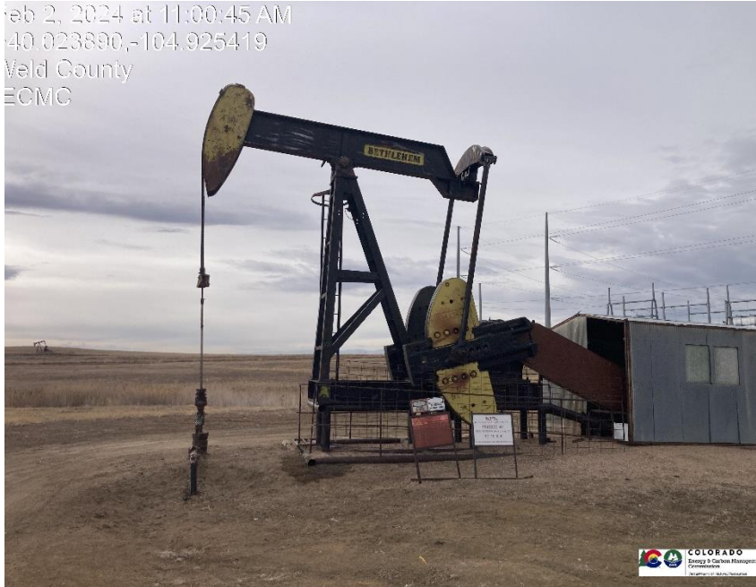
Pic 1 wellhead / pumpjack
