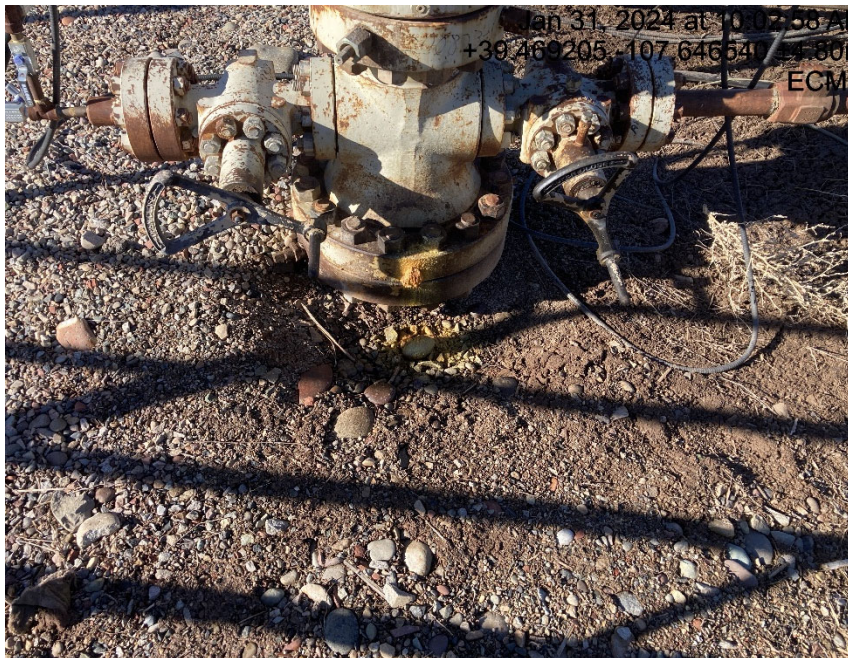
Well head leaking
