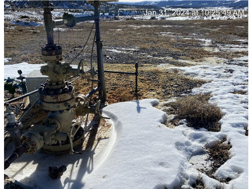
Oily waste on the ground out from wellhead
