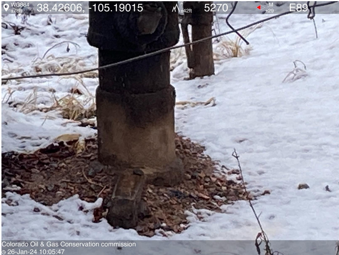
PHOTO 5: Bradenhead inaccessible or not visible. Install appropriate fittings to allow bradenhead visual inspection as per Rule 419.a.(1), (2). THIS IS THE SECOND NOTICE, IMMEDIATE ACTION IS REQUIRED.
