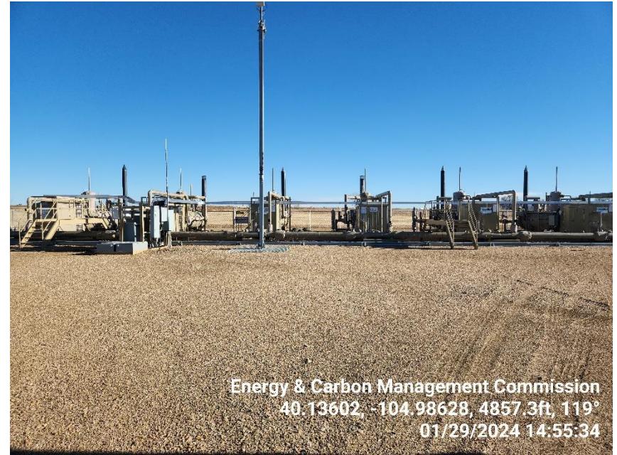
Photo 4 Horizontal Heated Separators.
