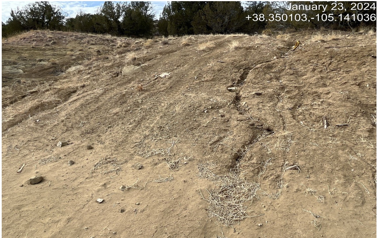
Photo 21. Facing toward the cut slope which still has signs of erosion rilling.
