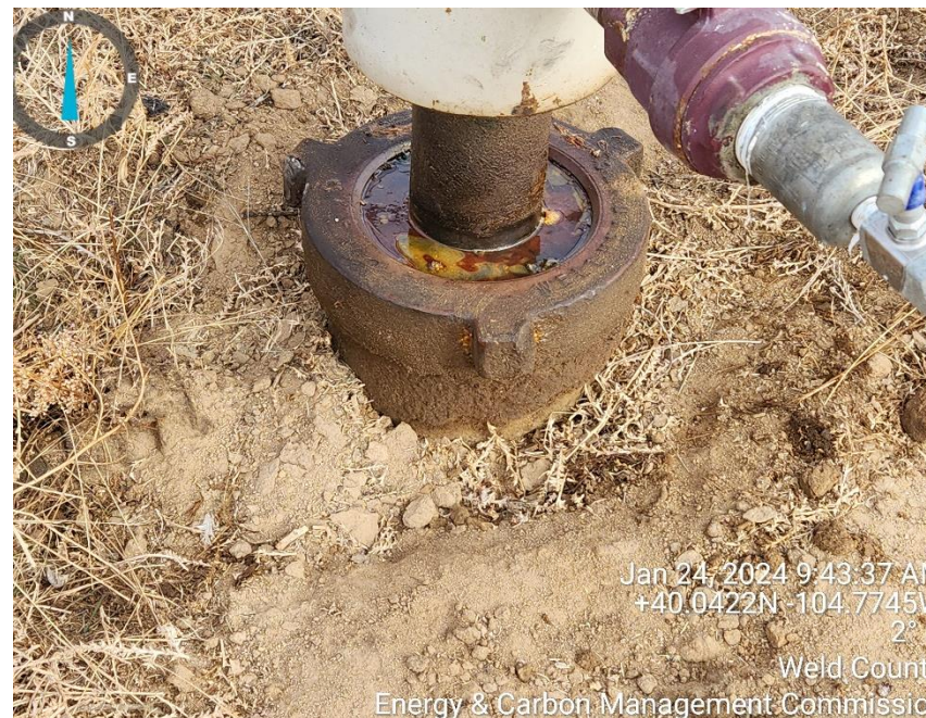
Photo 4 braden head leak
