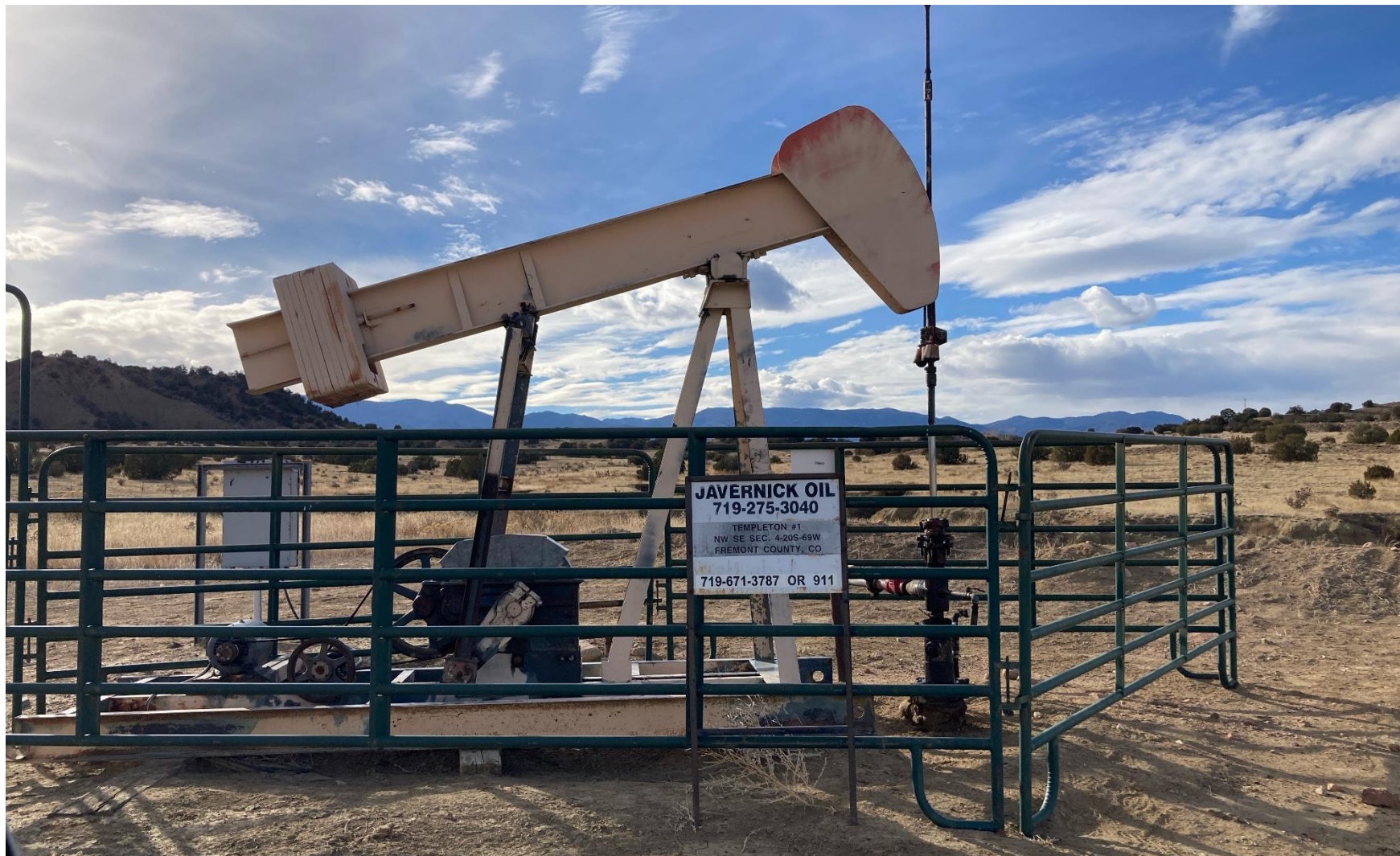
PHOTO 3: WELLHEAD AND EQUIPMENT
