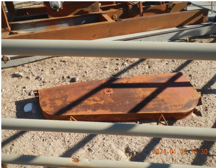
3. Belt guard on ground inside fencing.
