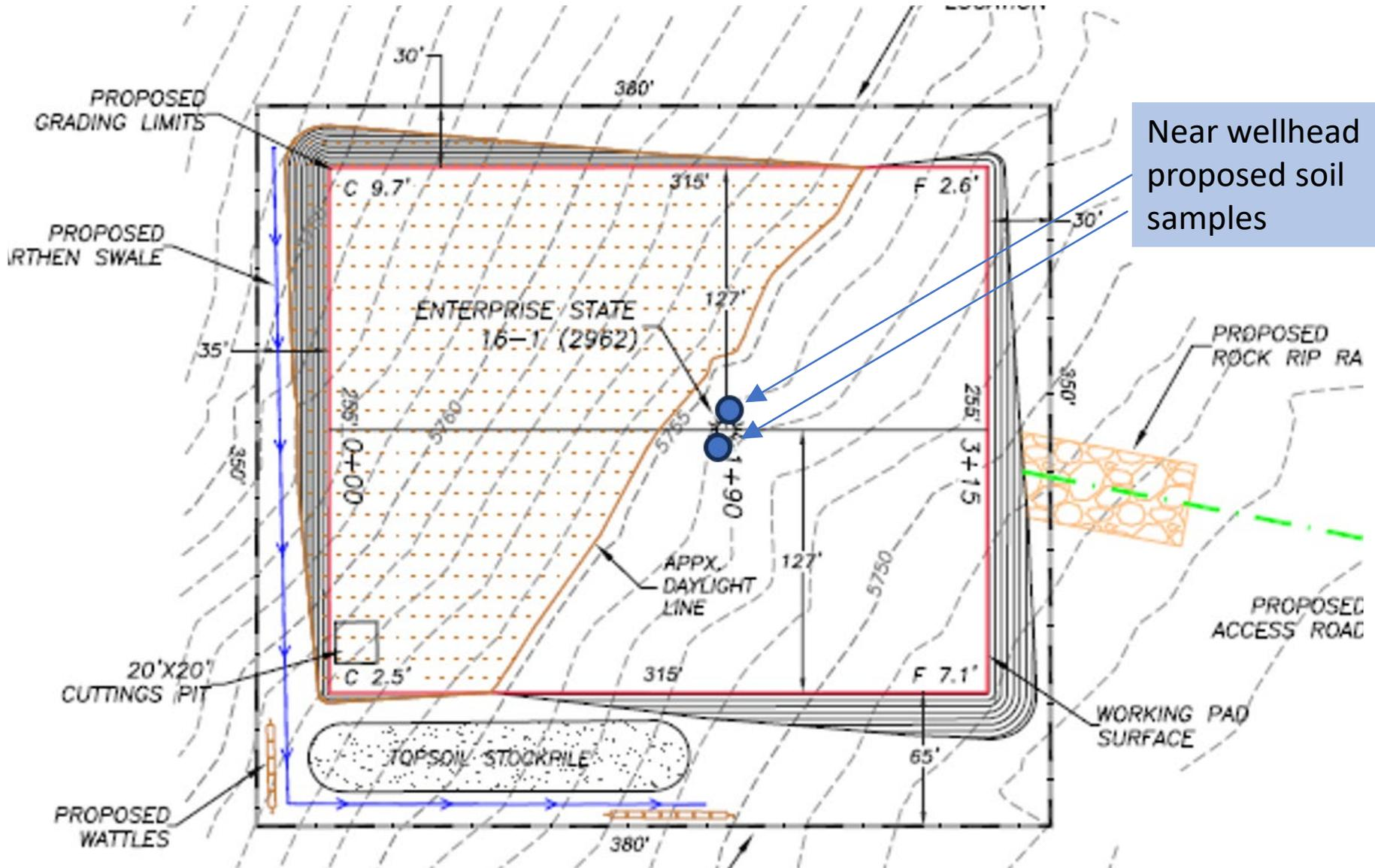
Near wellhead proposed soil samples
