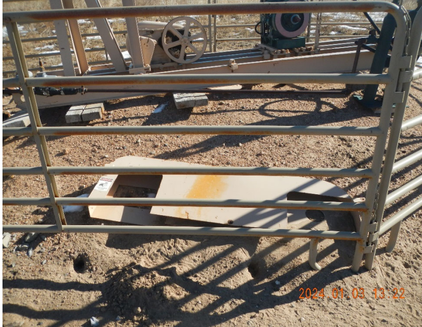
3. Belt guard inside well fencing on ground.
