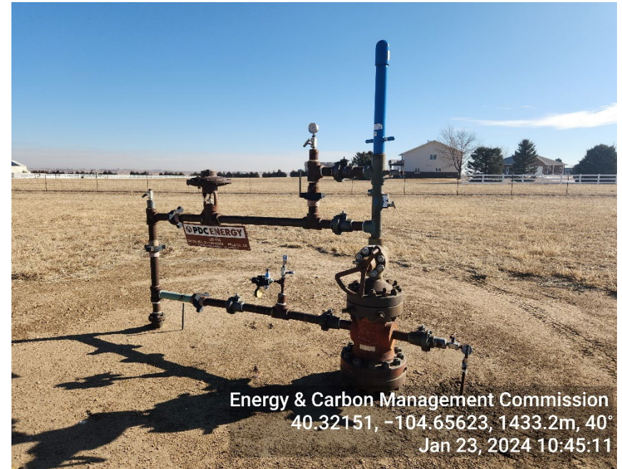
Photo 6: SI Wellhead
