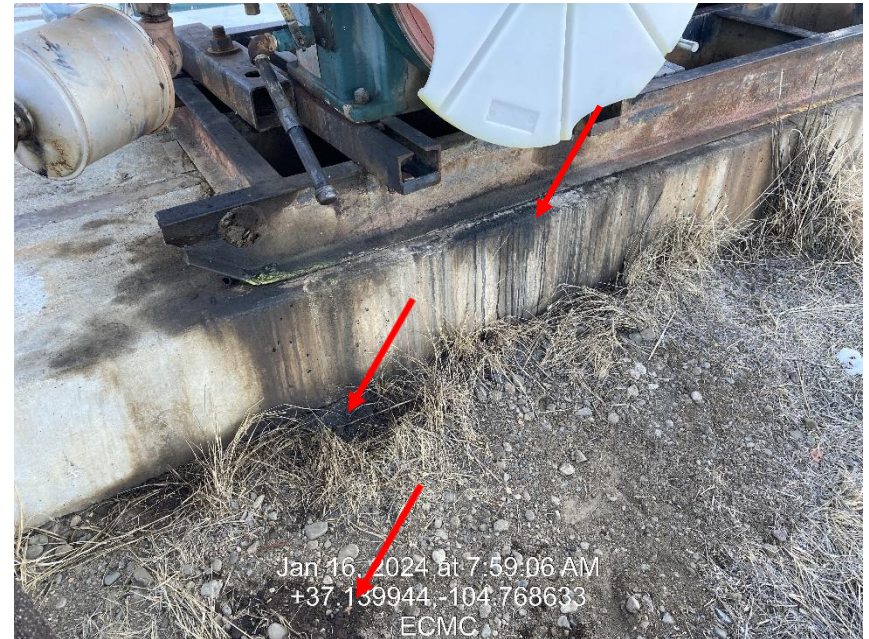
Photo 6 – Oil Leaking from Pumping Unit. Cement block/base and native ground are impacted.
