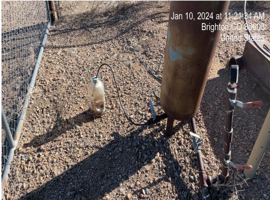
Photo 3. Photo taken of container used to collect oil, not contained or secure. Photo taken facing northeast.
