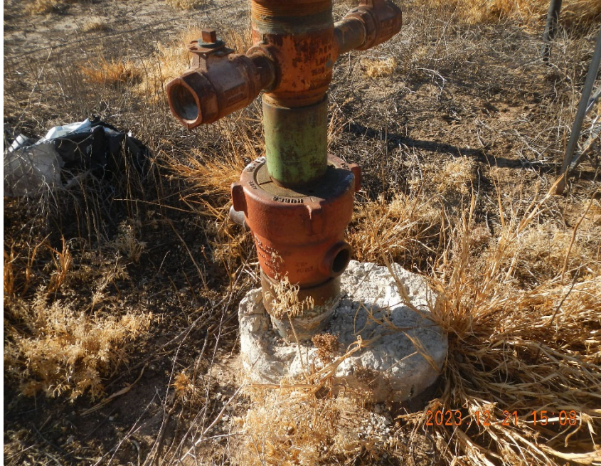
3. Surface casing missing plug.
