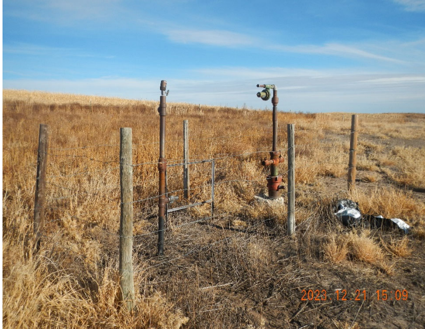
5. Flowline riser at wellhead area with open ended T connection.
