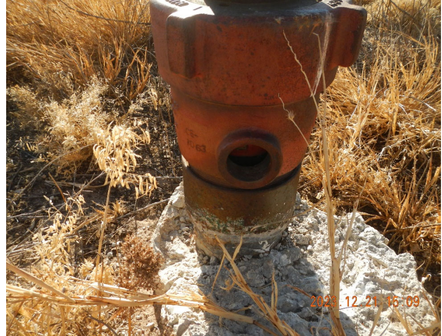
4. Closer view of surface casing open port.
