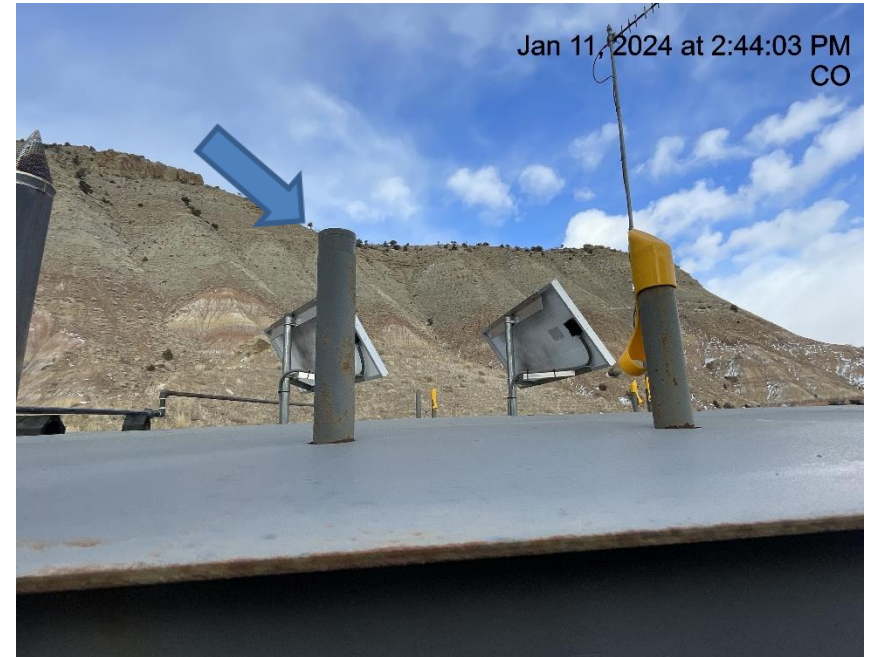
Photo # 2603 PRV vent line lacks cap
