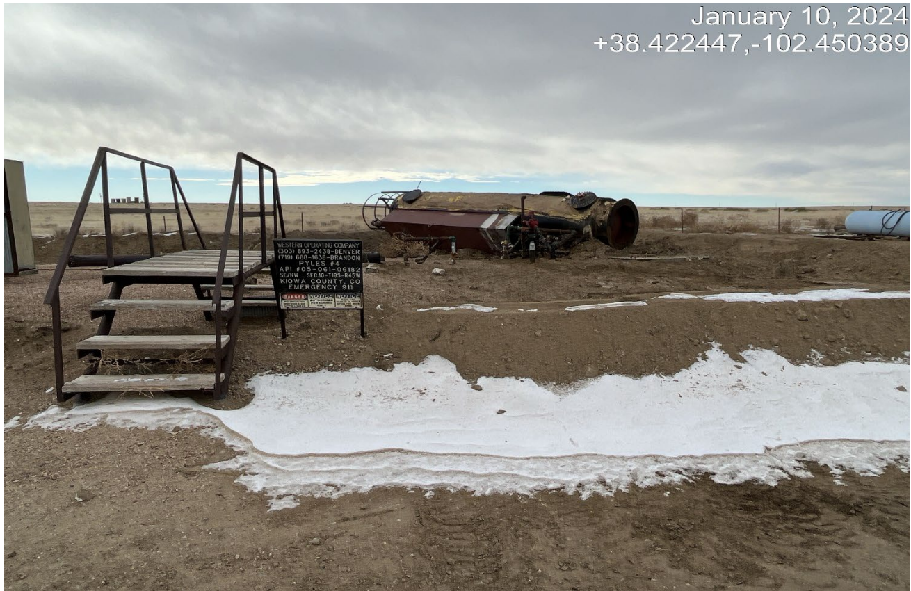
Photo 6. Facing toward the vertical heater treater which has fallen over and had a recent fire.
