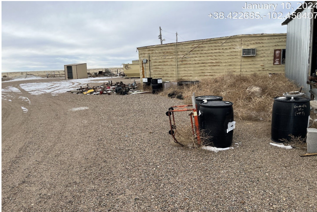
Photo 13. There are several chemical barrels on location with faded labeling and no secondary containment. Various pipe, supplies, and debris stored on location.
