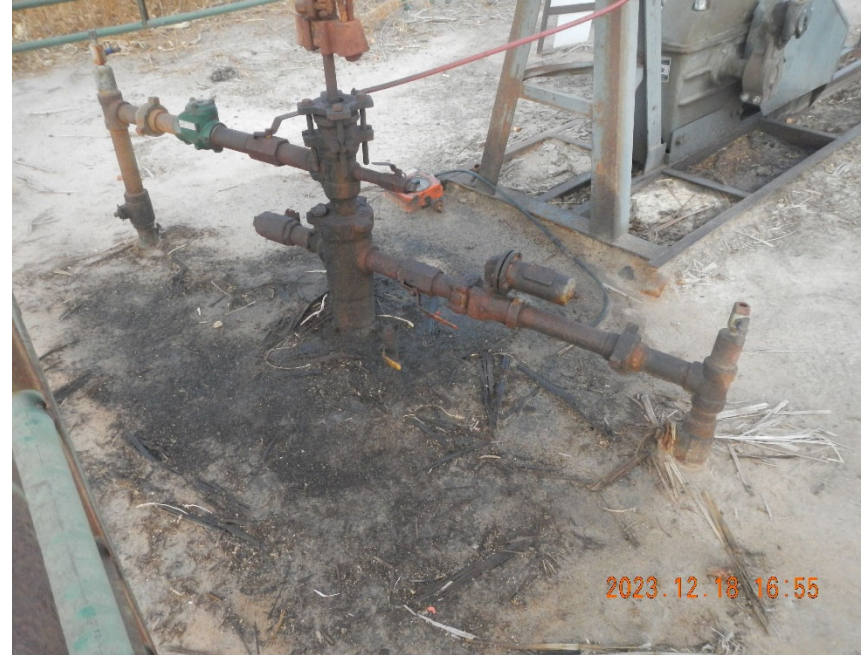
2. View of wellhead. Note stained soils around wellhead.
