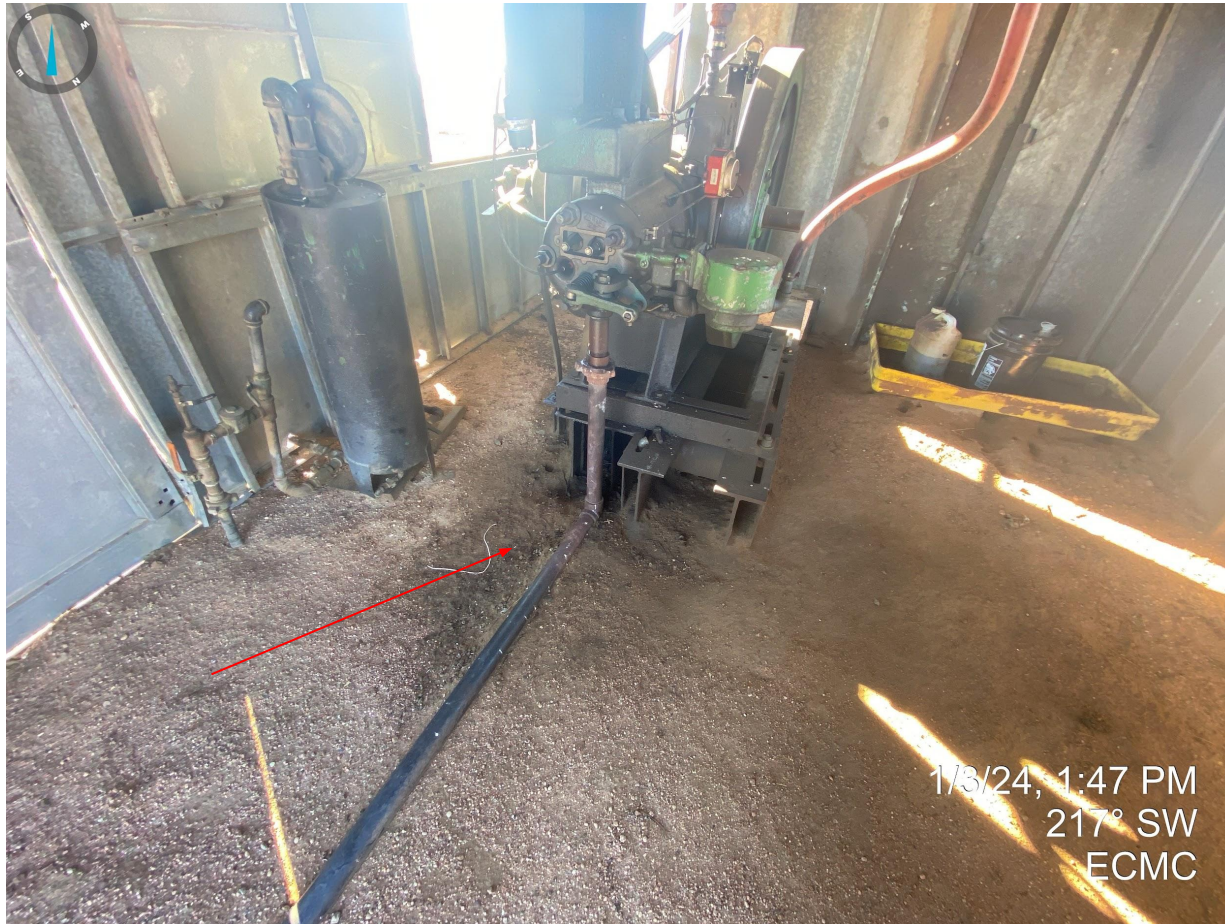
Photo 2. Stained soil observed at the pumpjack motor.
