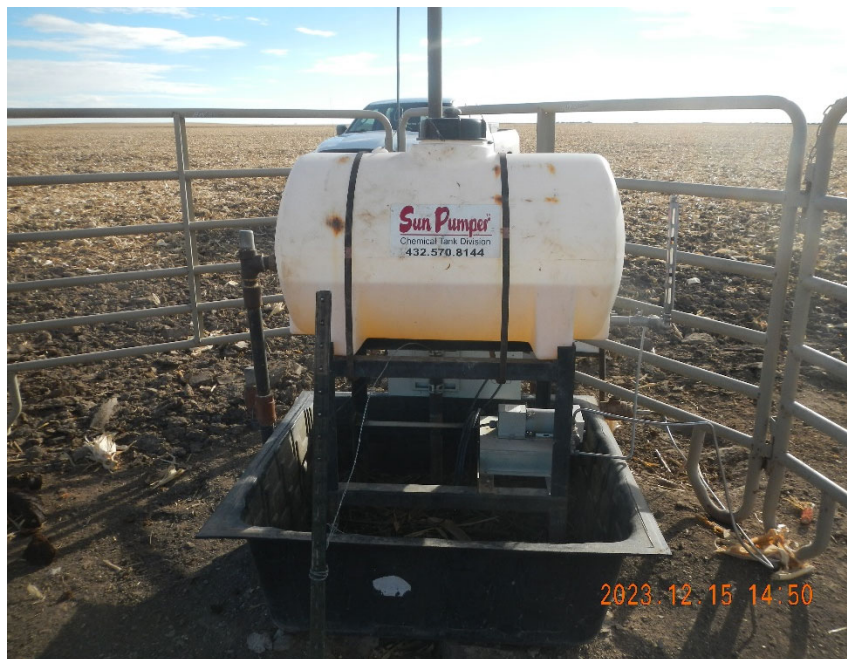
3. Chem tank and pump at wellhead.
