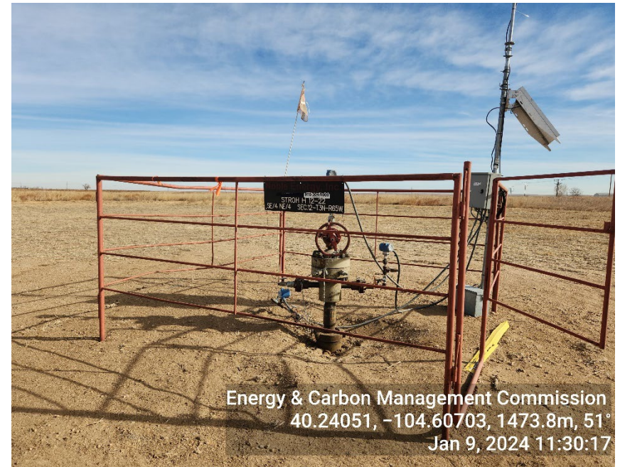
Photo 1: TA Wellhead
