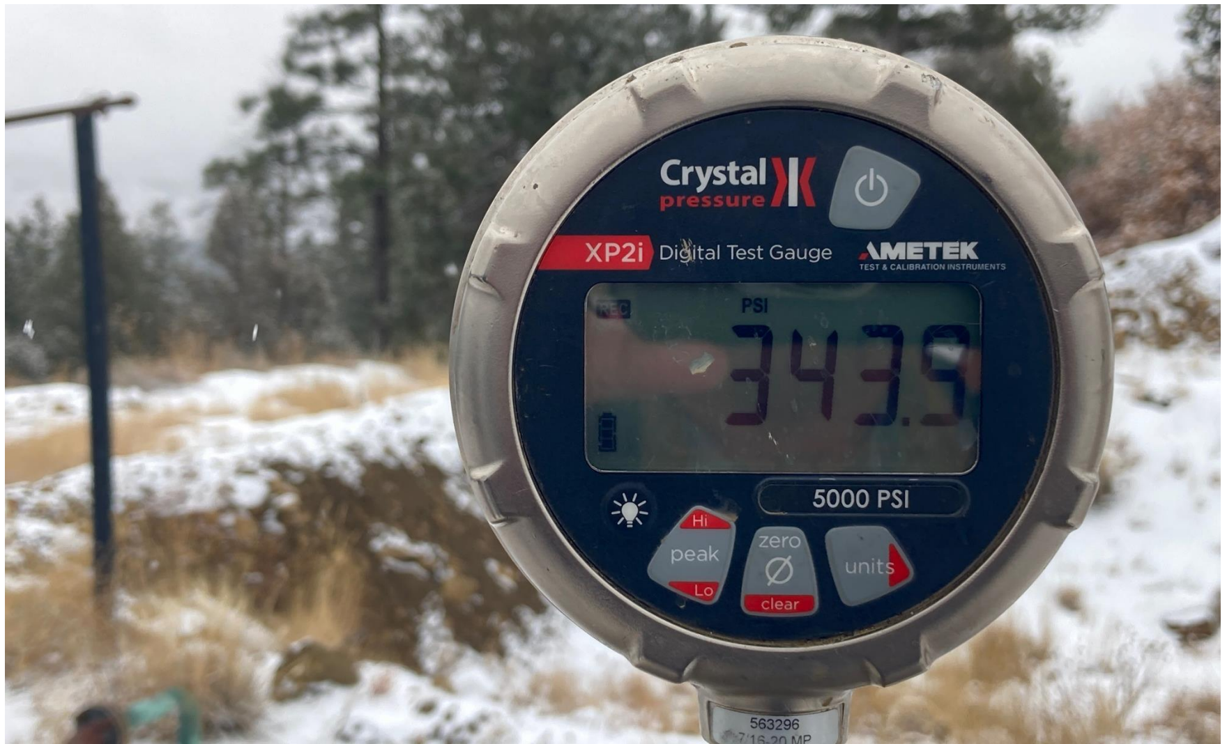
PHOTO 7: 15 MIN. FINAL MIT PSI 343.9, TOTAL -.9 LOSS DURING 15 MIN. MIT, -.1 LOSS IN LAST 5 MIN. OF MIT.
