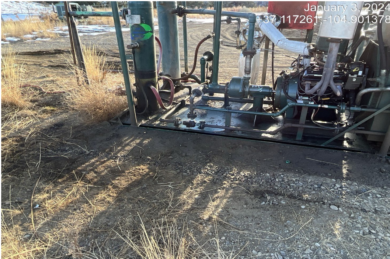
Photo 3. The engine skid has oil and has spilled out onto the ground.
