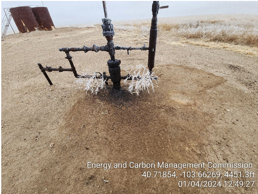
Photo 3 – Wellhead – Stained Soil
