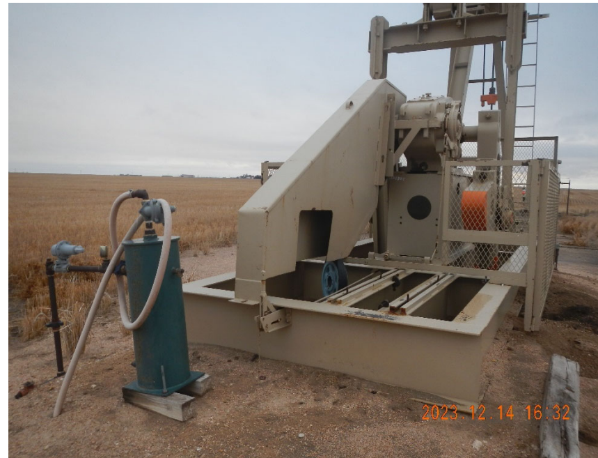
4. Prime Mover removed. Supply gas dehydrator.
