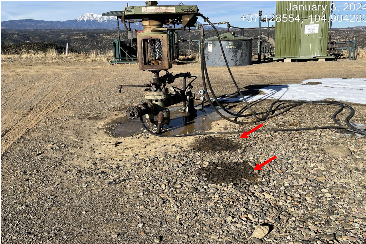
Photo 1. There are two spots of oil stained gravel neat to the wellhead.
