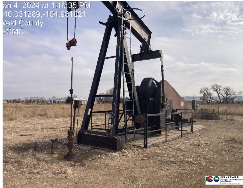
Pic 1 wellhead / pump jack / Electric
