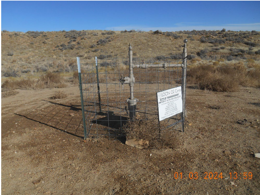
Wellhead with fencing and sign
