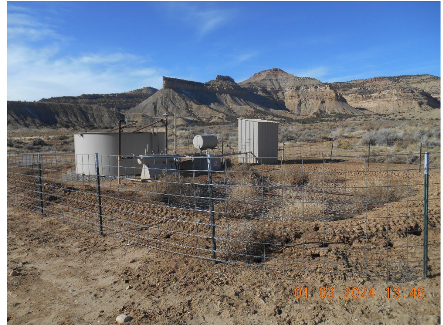
Tank Battery and Separator, Meter Housing and blowdown pit with fence and berms
