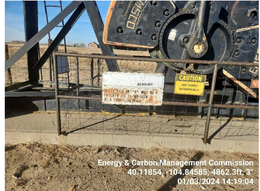
Photo 2 WH sign faded and needs replaced.
