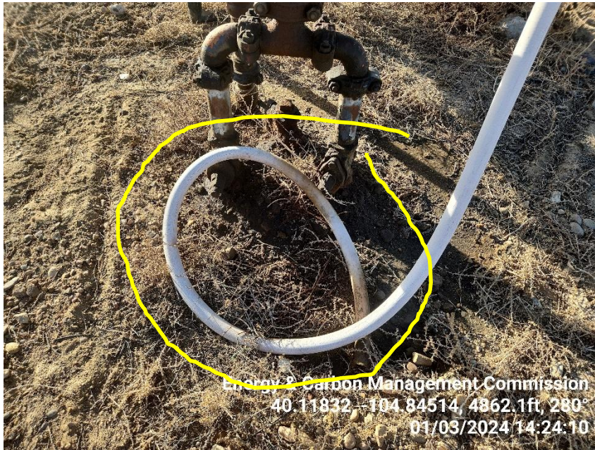
Photo 11 Stained soil by the flow line manifold.
