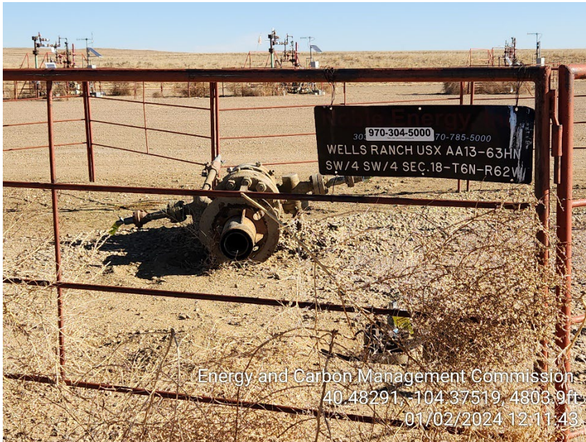
Photo 3 – Unused Wellhead Tree
