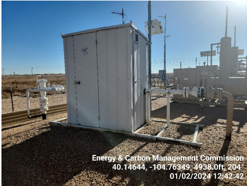
Photo 13 Gas Meter Run, card indicates current calibration.
