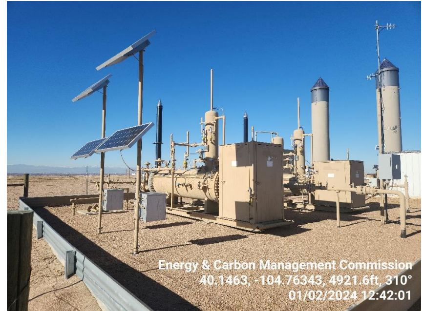
Photo 10 Horizontal Heated Separators.
