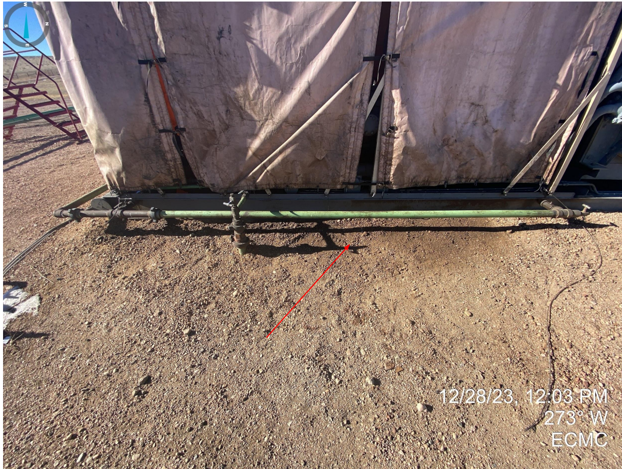
Photo 1. Stained soil observed around compressor station.
