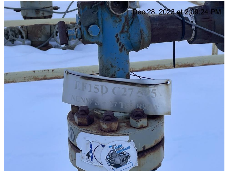
Photo # 1367 Wellhead sign lacks required info
