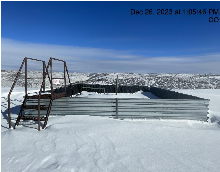
Photo # 852 Tank battery lacks signage
