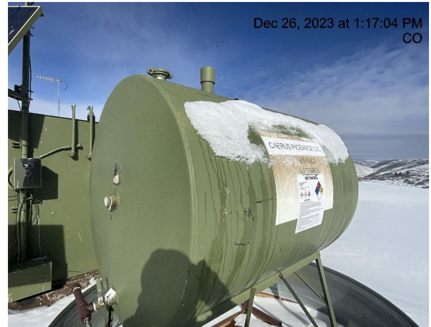
Photo # 847 Methanol tank missing required info
