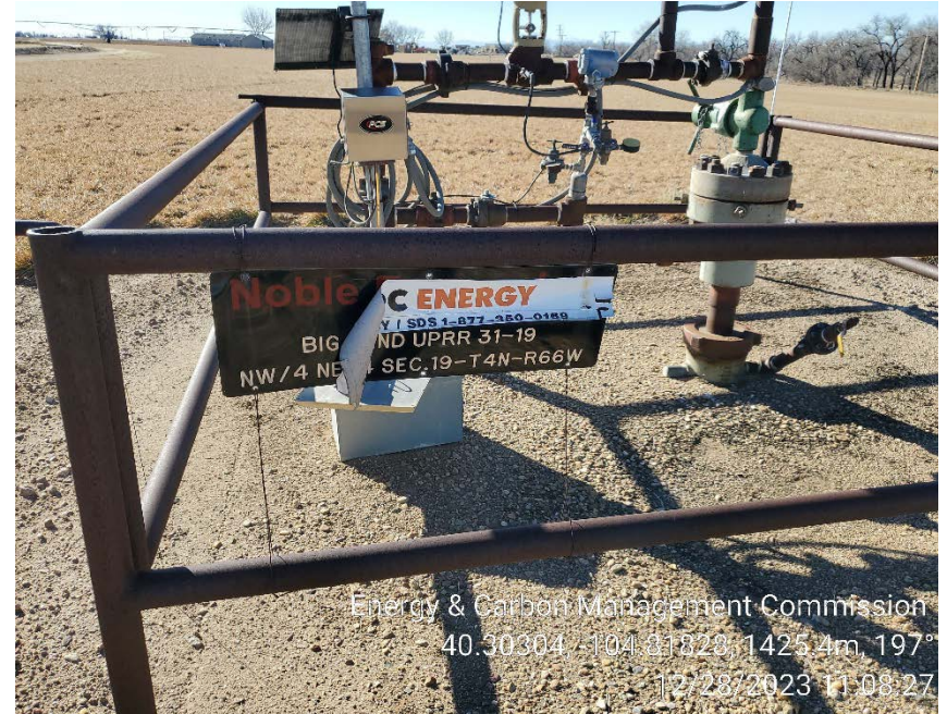
Wellhead producer and emergency contact number decals
