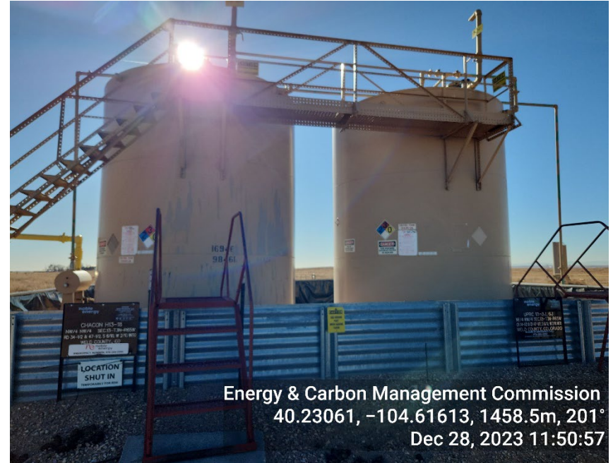
Photo 2: Centralized Tank Battery
