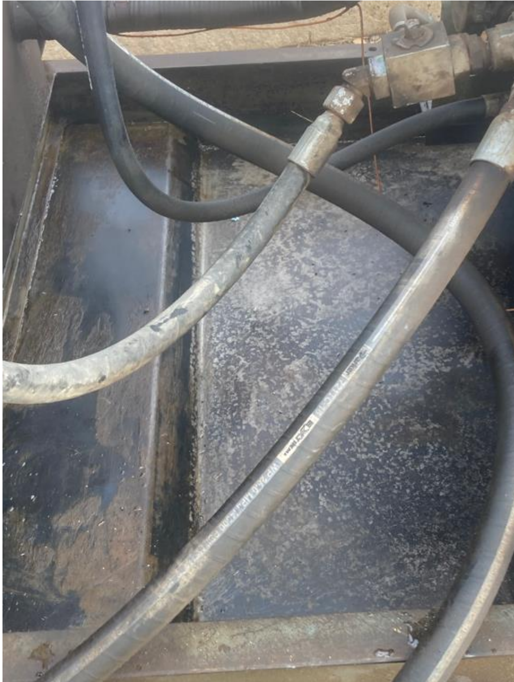
PHOTO 1: THE OILY WASTE IN THE ENGINE SKID HAS BEEN REMOVED AND MECHANICAL MAINTENANCE PERFORMED. THE SOIL STAINS AROUND THE SKID HAVE ALSO BEEN REMOVED AND THE SELF INSPECTION PROCESS REVIEWED.
