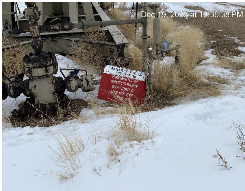
Wellhead sign missing required information
