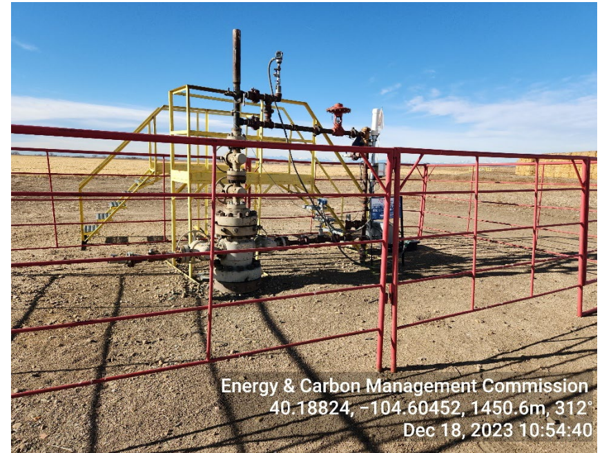
Photo 4: SI Wellhead
