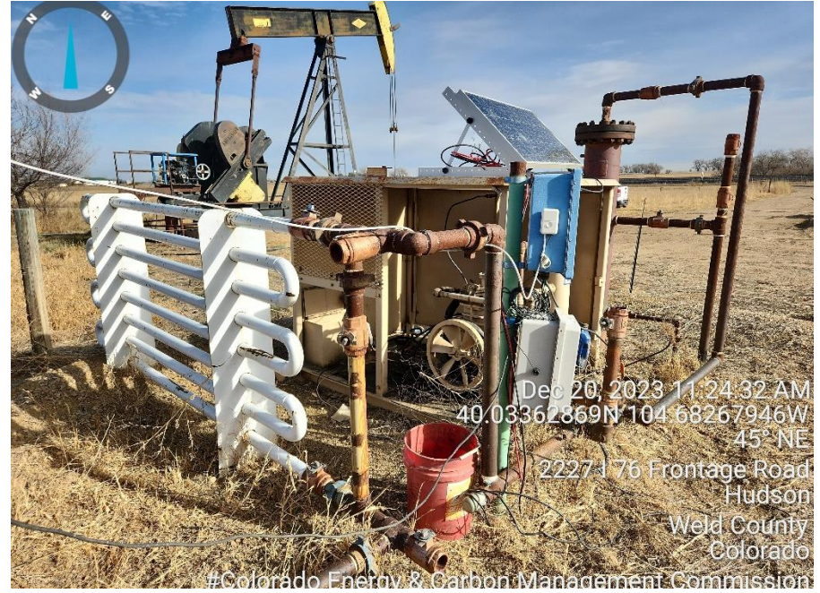
Photo 4 Unused equipment pump in disrepair and no motor, Stained soil around unit.
