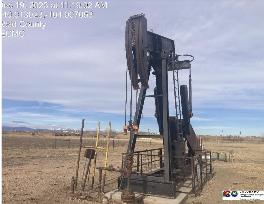
Pic 1 wellhead / pump jack
