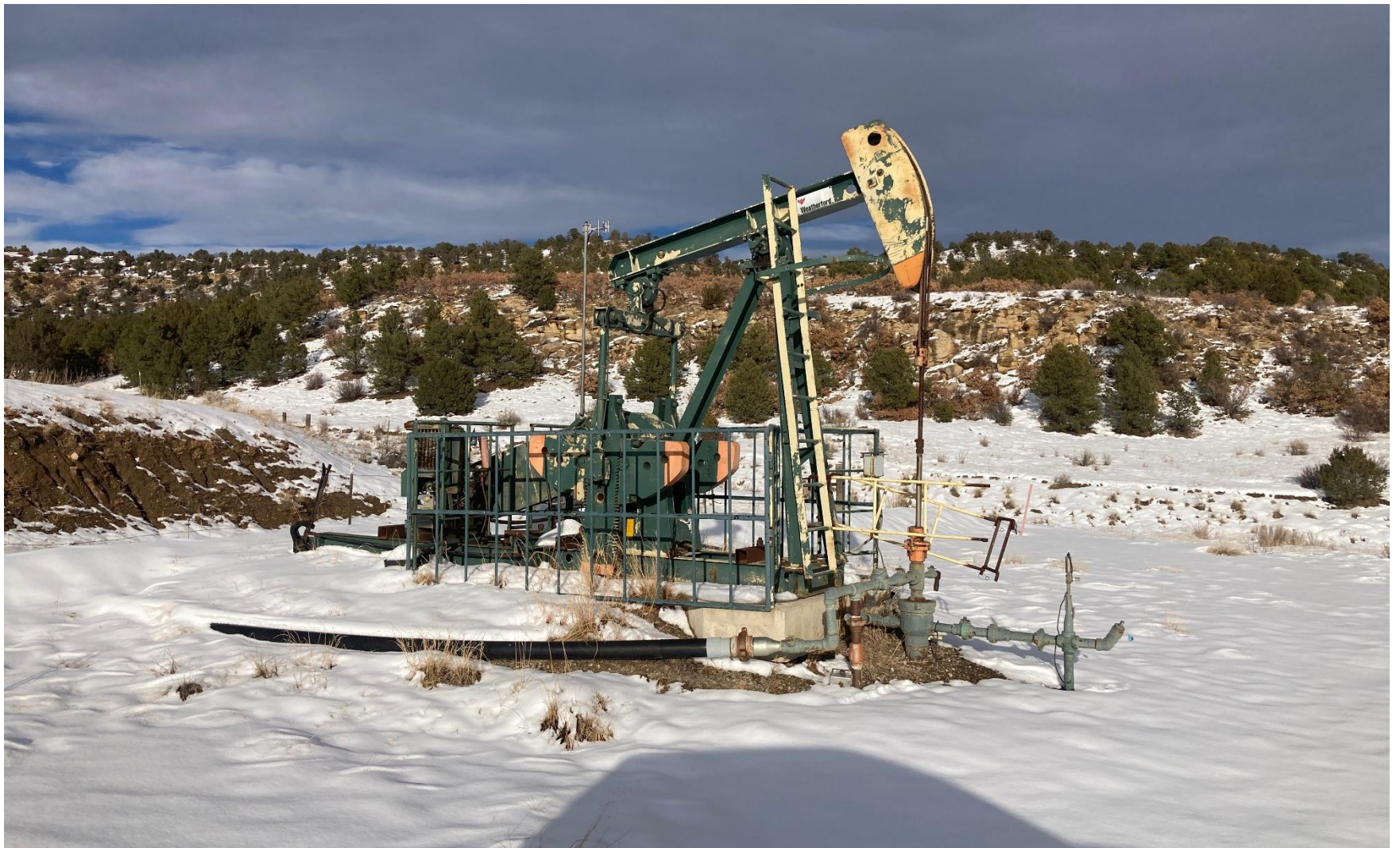
PHOTO 3: WELLHEAD AND EQUIPMENT
