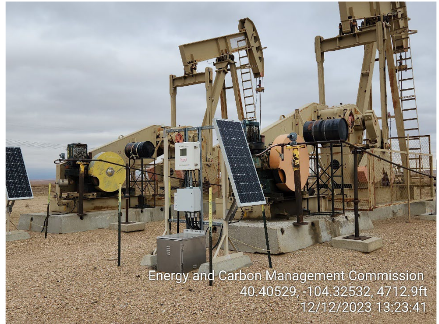
Photo 8 – Gas Engines
