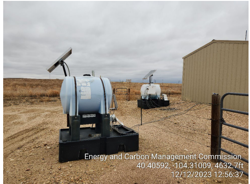
Photo 4 – Chemical Containers missing Labels
