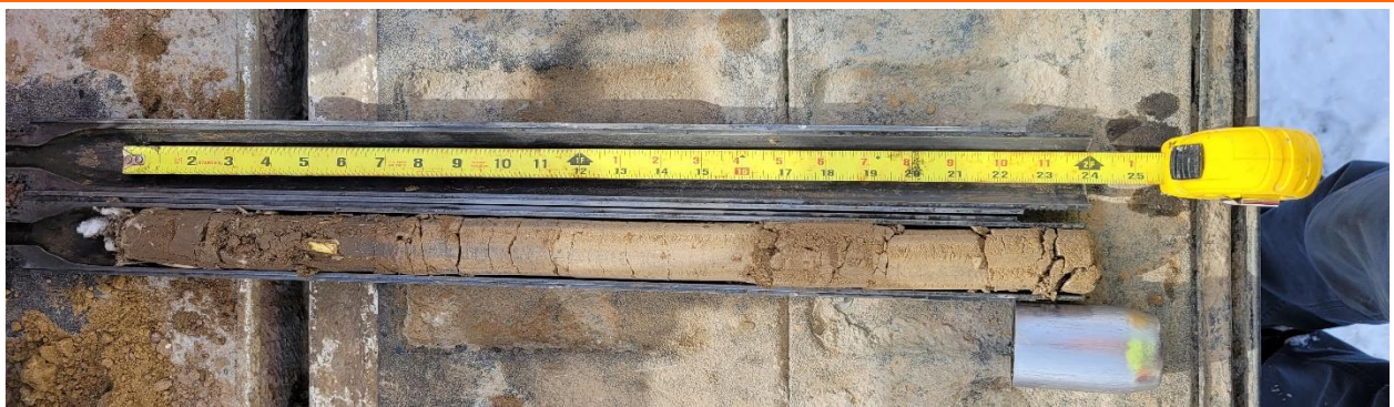
B-2 at 0 feet. Topsoil thickness of about 11 inches
