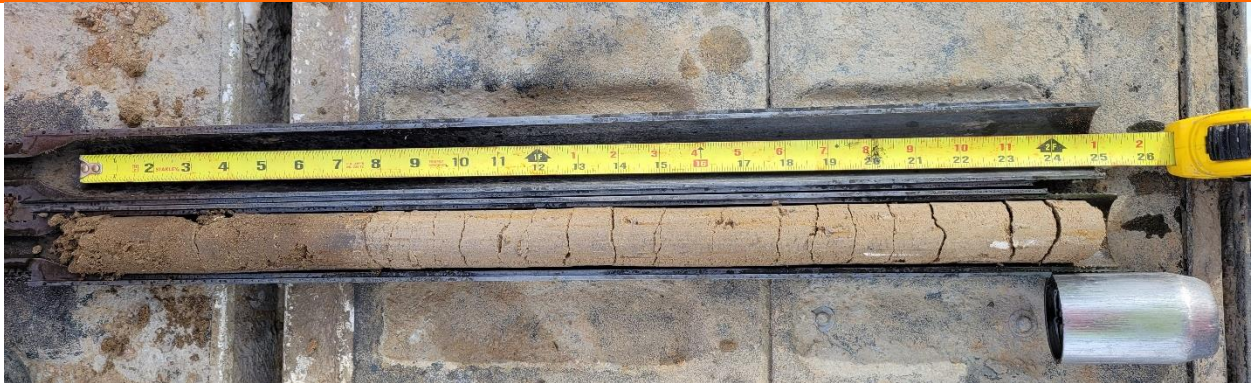
B-2 at 0 feet. Topsoil thickness of about 8 inches
