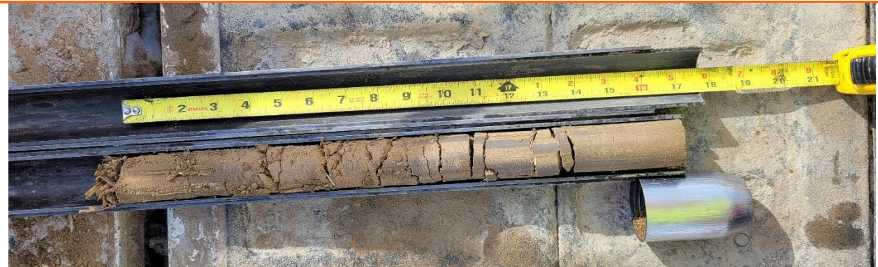
B-1 at 0 feet. Topsoil thickness of about 6½ inches
