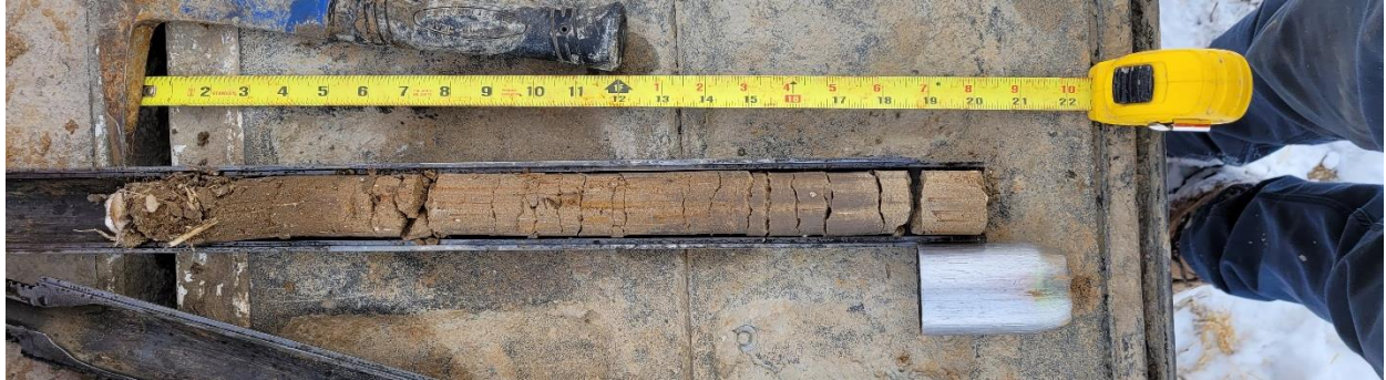
B-1 at 0 feet. Topsoil thickness of about 5½ inches
