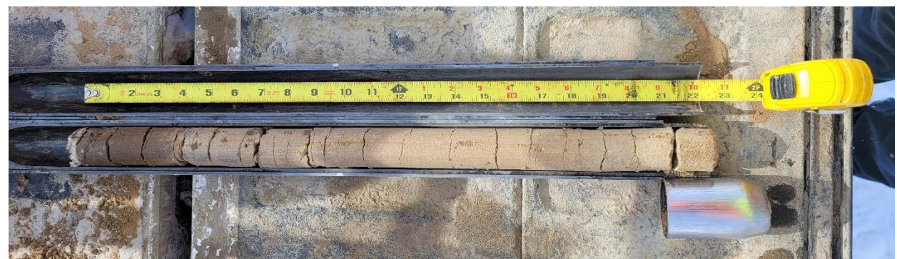
B-3 at 0 feet. Topsoil thickness of about 7½ inches
