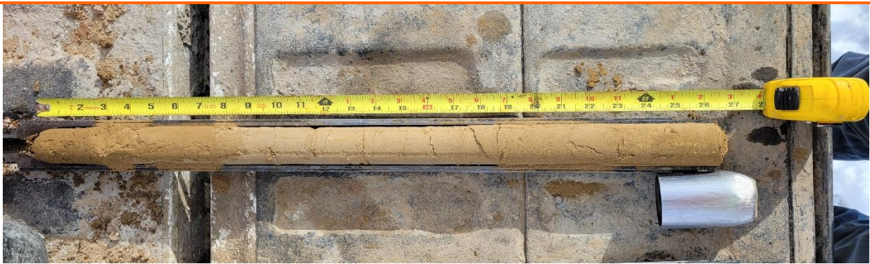
B-3 at 0 feet. Topsoil thickness of about 7½ inches
