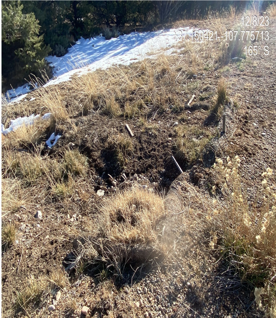
Photo 3. View of failing storm water BMPs and additional rill erosion forming in the eastern interim reclamation area.
