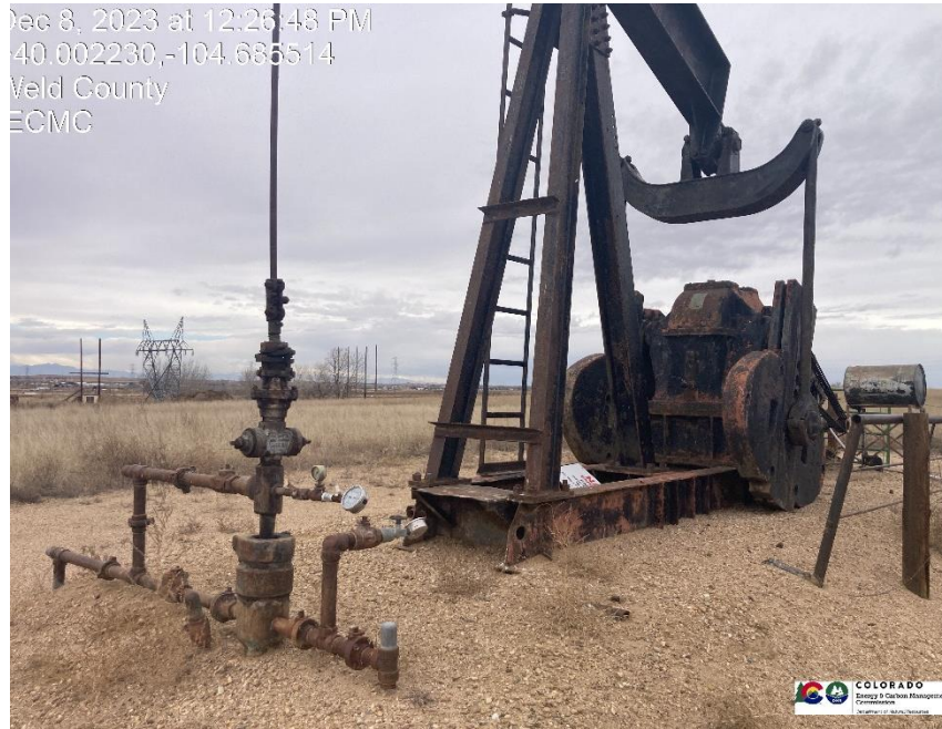
Pic 1 wellhead
